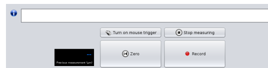
Figure 2.2: Measuring control panel. The number of digital displays will vary between 1 and 3 depending on what type of measuring platform hardware you have.
